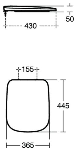
Dimensions: All measurements are in millimetres and are subject to normal manufacturing variations.
