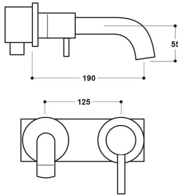
Dimensions: All measurements are in millimetres and are subject to normal manufacturing variations.
