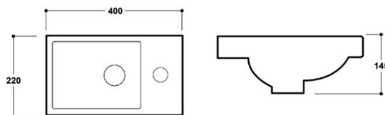
Dimensions: All measurements are in millimetres and are subject to normal manufacturing variations.
