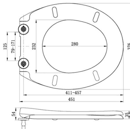
Dimensions: All measurements are in millimetres and are subject to normal manufacturing variations.
