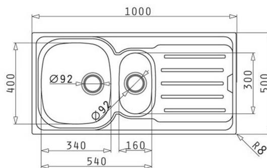
Dimensions: All measurements are in millimetres and are subject to normal manufacturing variations.
