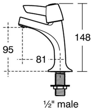
Dimensions: All measurements are in millimetres and are subject to normal manufacturing variations.
