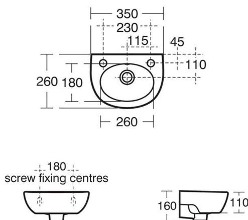
Dimensions: All measurements are in millimetres and are subject to normal manufacturing variations.
