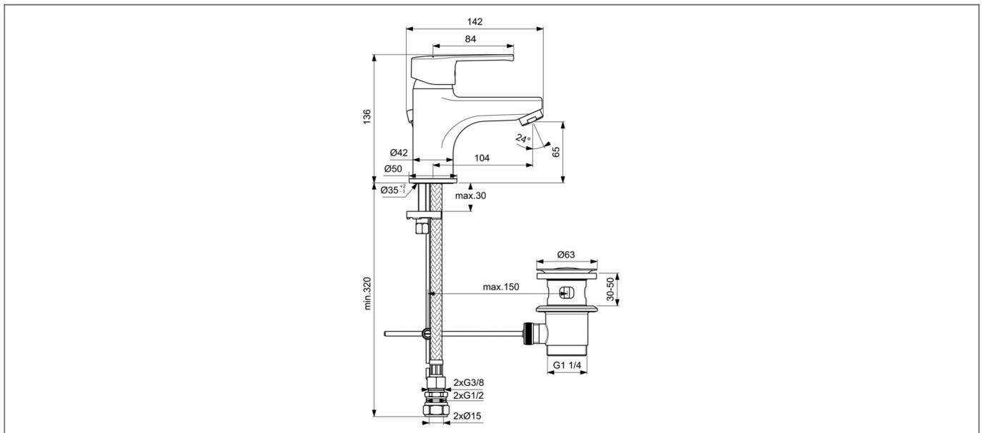
Dimensions: All measurements are in millimetres and are subject to normal manufacturing variations.
