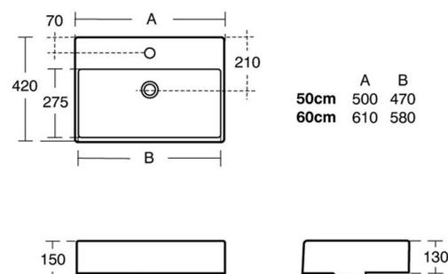
Dimensions: All measurements are in millimetres and are subject to normal manufacturing variations.
