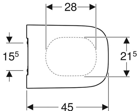
Dimensions: All measurements are in millimetres and are subject to normal manufacturing variations.
