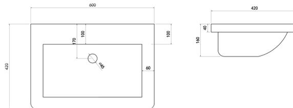
Dimensions: All measurements are in millimetres and are subject to normal manufacturing variations.
