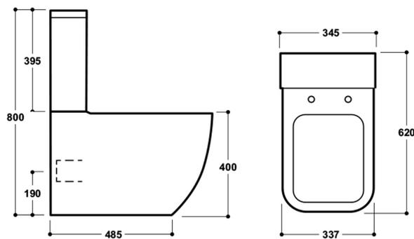
Dimensions: All measurements are in millimetres and are subject to normal manufacturing variations.
