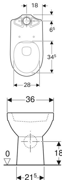
Dimensions: All measurements are in millimetres and are subject to normal manufacturing variations.
