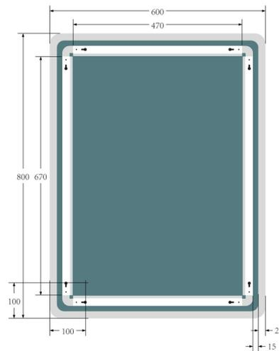
Dimensions: All measurements are in millimetres and are subject to normal manufacturing variations.
