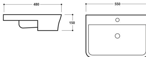
Dimensions: All measurements are in millimetres and are subject to normal manufacturing variations.
