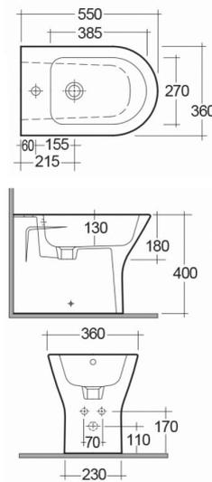
Dimensions: All measurements are in millimetres and are subject to normal manufacturing variations.
