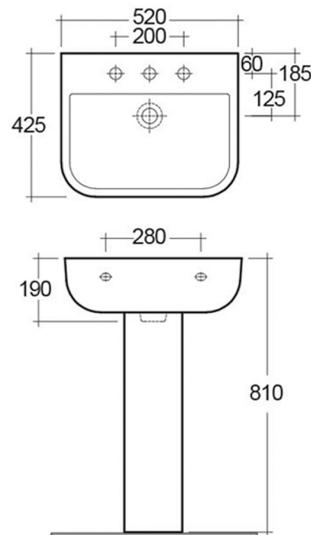
Dimensions: All measurements are in millimetres and are subject to normal manufacturing variations.
