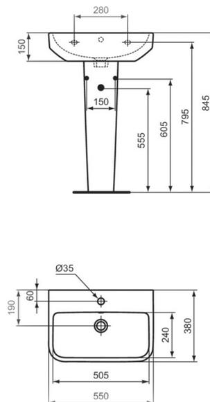
Dimensions: All measurements are in millimetres and are subject to normal manufacturing variations.
