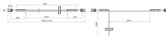
Dimensions: All measurements are in millimetres and are subject to normal manufacturing variations.
