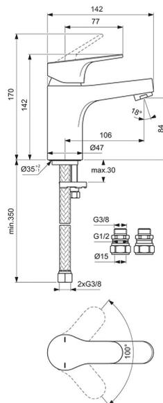
Dimensions: All measurements are in millimetres and are subject to normal manufacturing variations.
