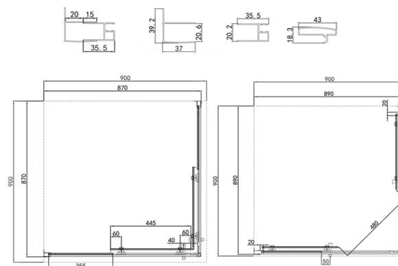
Dimensions: All measurements are in millimetres and are subject to normal manufacturing variations.
