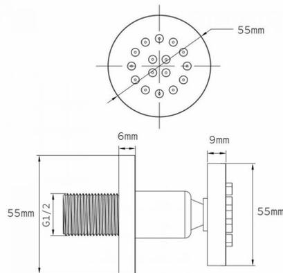
Dimensions: All measurements are in millimetres and are subject to normal manufacturing variations.
