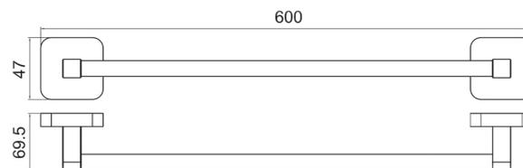
Dimensions: All measurements are in millimetres and are subject to normal manufacturing variations.
